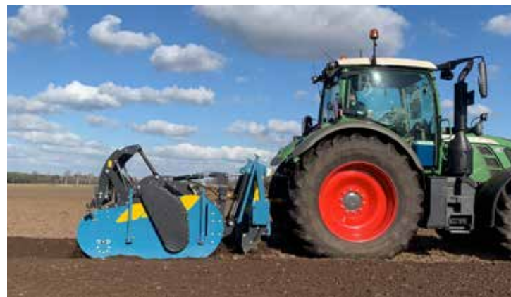
▲ Culter in combination with a spading machine.
